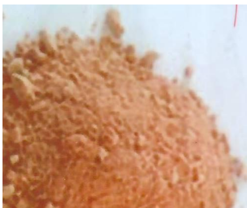
Fig. 2. Mixture of polycrystalline powders with nanostructured BAF-1 and BAF-2
